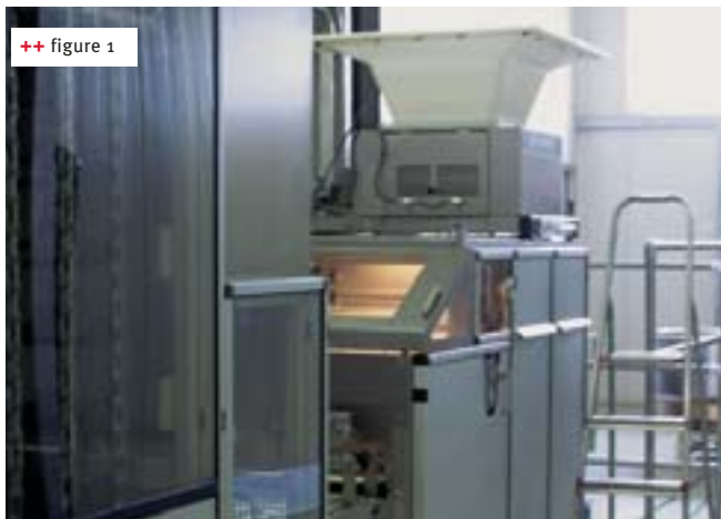
++ figure 1 A classical dough divider is responsible for dough portioning
